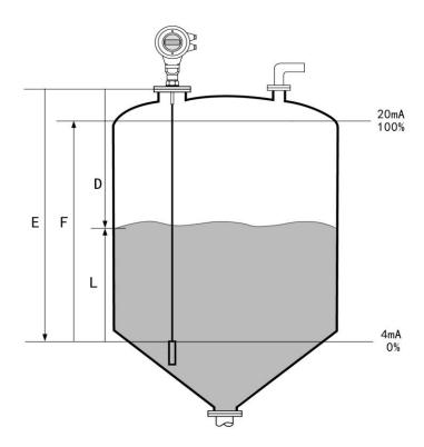
Reflection of the pulse signal along the cable type or bar type probe to the instrument electronic circuit part, microprocessor to signal processing, identify the microwave pulse produced by the echo in the material surface. Correct echo signal recognition by the pulse software complete, distance material on the surface of the distance D is proportional to the pulse travel time T:
